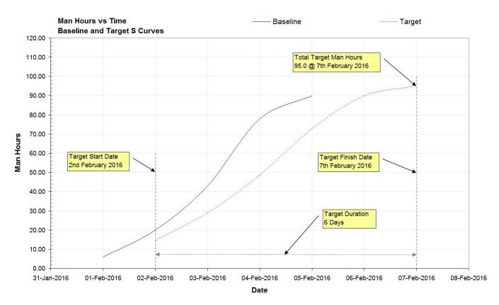
Figure 2: Target S Curve (Showing Baseline S Curve For Comparison)
