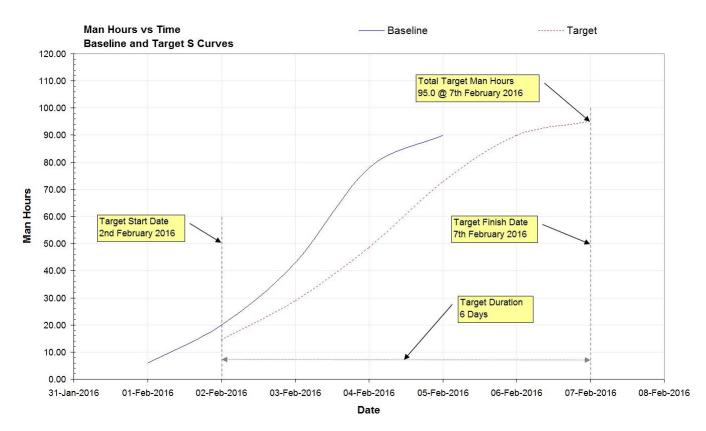
Figure 13: Target Man Hours versus Time S Curve (Showing Baseline S Curve For Comparison)
