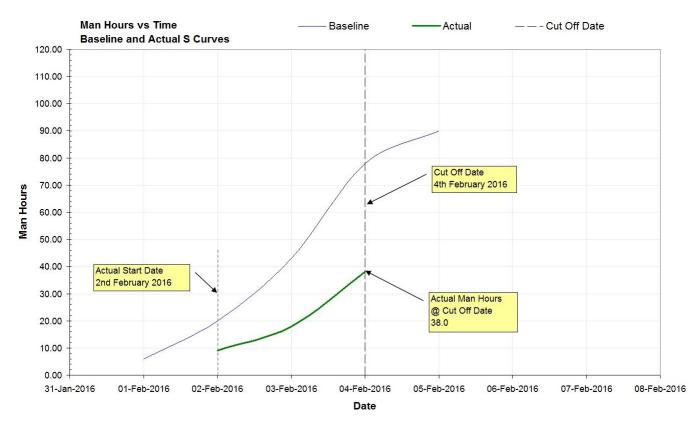
Figure 3: Actual S Curve (Showing Baseline S Curve For Comparison)
